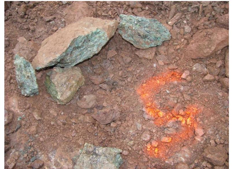
FIG 4 SAMPLE COLLECTED AT GOSHEN MAIN (~ 4% COPPER)
